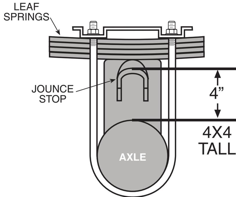
On some models with the tall jounce bumper stop, the lower bracket will have to be modified to fit level with the axle.
