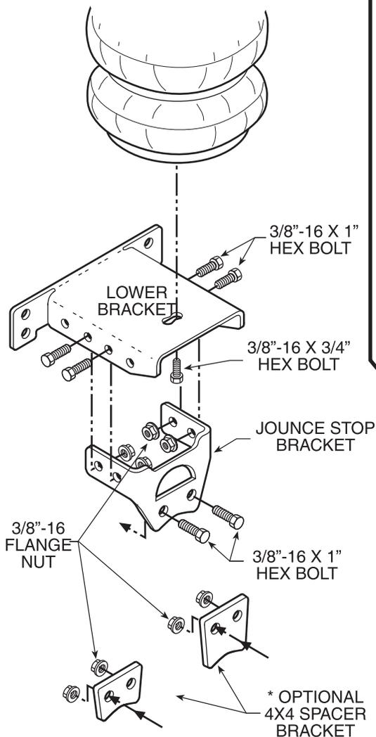
**\*NOTE:** AN ADDITIONAL SPACER MAY BE NECESSARY FOR SOME 4X4's. IF THE SPACER IS REQUIRED, USE THE SPACER THAT BEST FITS THE VEHICLE.
